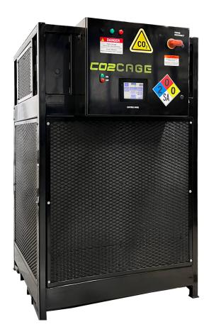
The  $\mathrm{CO_2Cage}$  serves as the primary source of supply to extractors with a capacity of 1,600 lbs of liquid  $\mathrm{CO_2}$ . It provides a safe and convenient solution for constant pressure input levels needed for efficient extraction, and incorporates sixteen 100-pound liquid  $\mathrm{CO_2}$  cylinders, DOT certified, attached to a single manifold.
